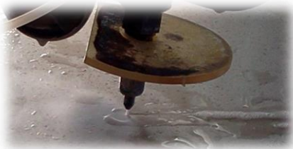
Cut-out by water jet
