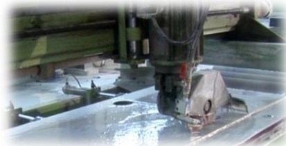
Cutting with bridge saw
